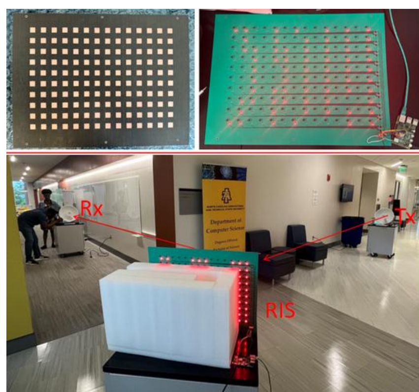
RIS hardware with 140 binary elements and the indoor test at NCAT
